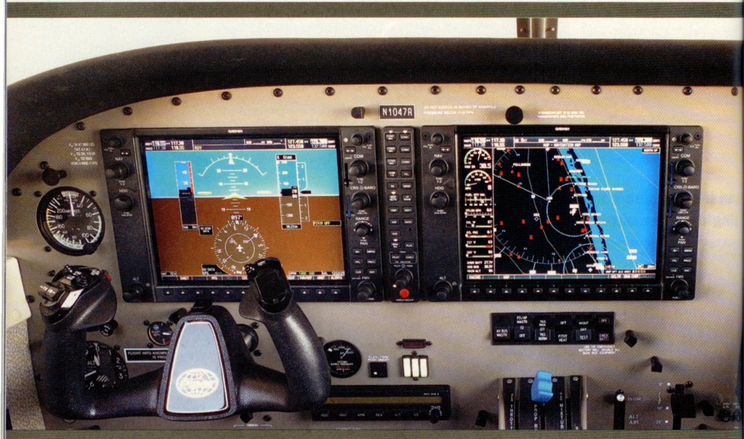
Starting this month, Saratoga buyers can opt for the Garmin G1000 cockpit, which still interfaces with the S-Tec autopilot, but the Garmin navigation and communications functions are integrated into the primary and multifunction displays.
