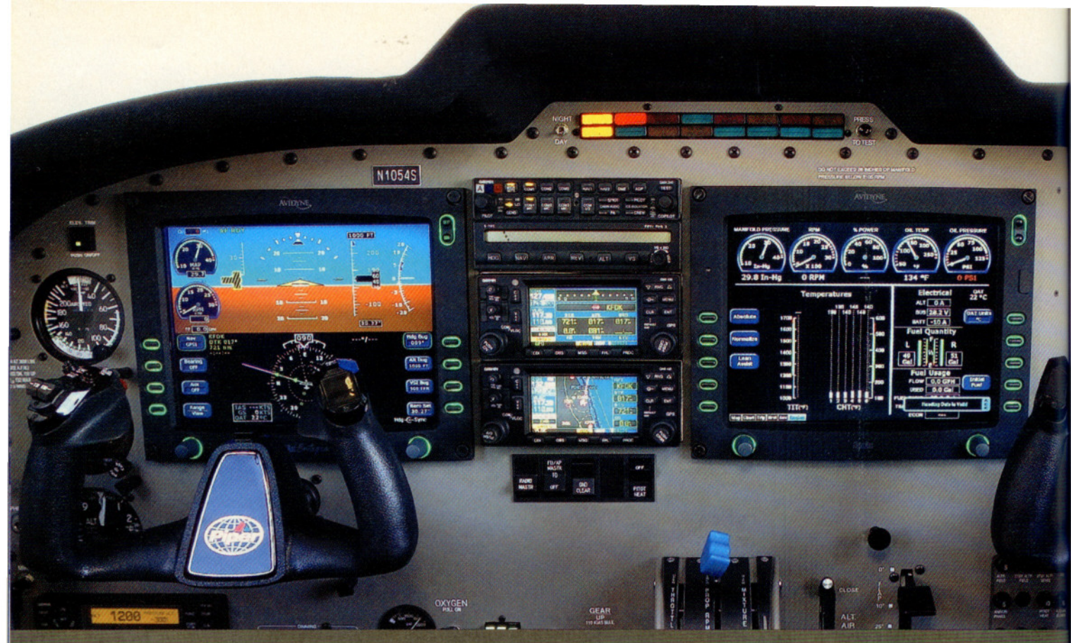
The Avidyne Entegra avionics system with its large primary and multifunction displays, combined with the Garmin 430s and S-Tec autopilot, provide a clutter-free panel and remarkable assistance to the pilot.
